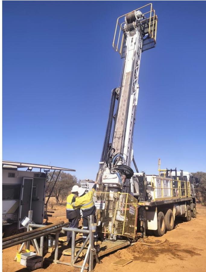
Figure (1): Diamond drill rig at the Montague-Boulder deep target.
