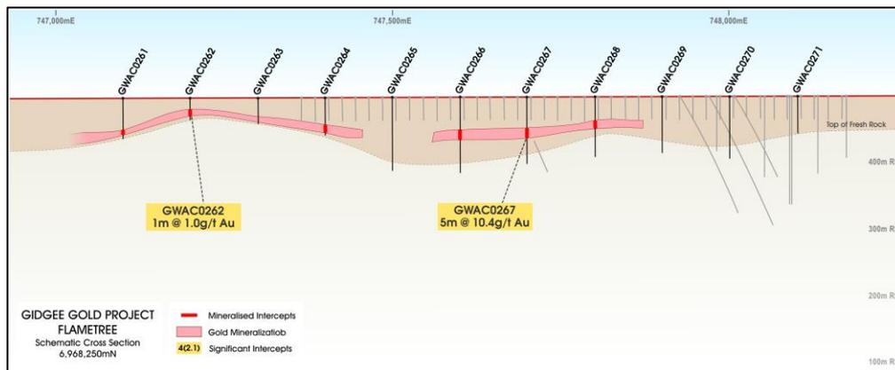
Figure (4): Flametree aircore drilling cross section 6,968,250mN
