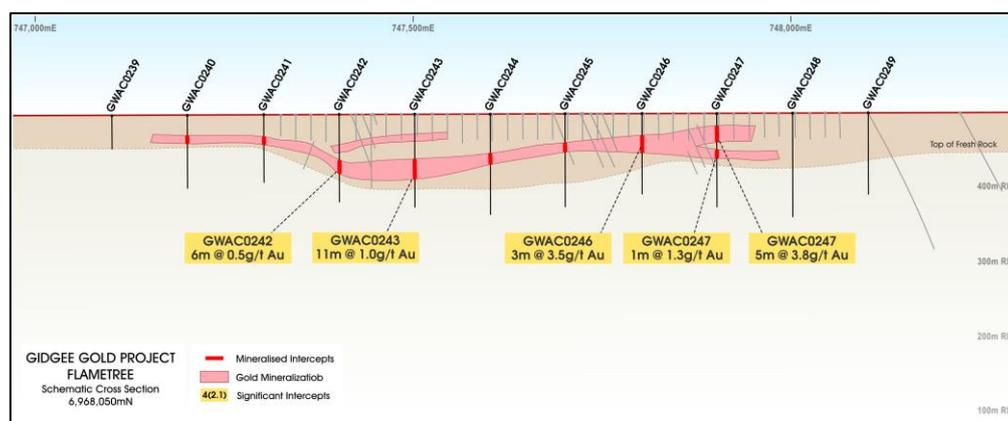
Figure (5): Flametree aircore drilling cross section 6,968,050mN
