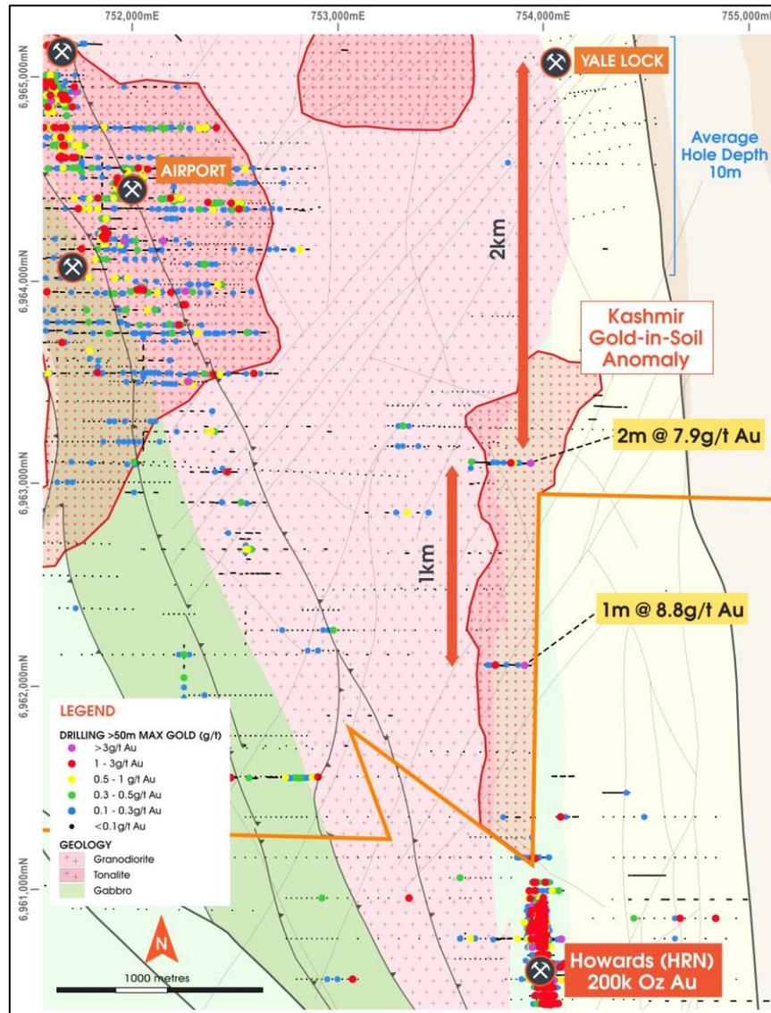
Figure (3): Kashmir prospect gold-in-soil anomaly and RC drill traverses from 2020 drilling
