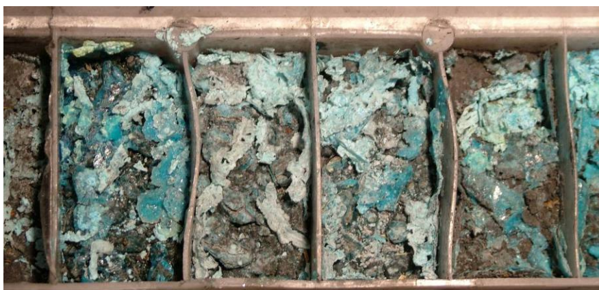
Copper sulphates leaching from chalcocite, CRC200 89 to 93m
