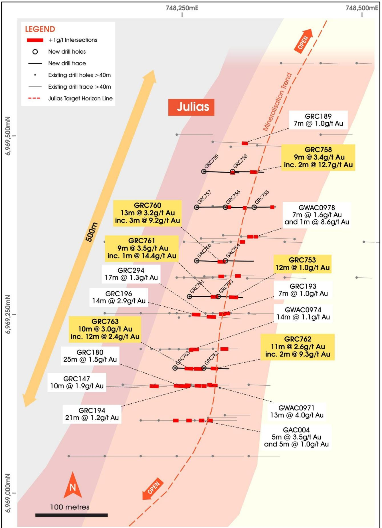
Figure (2): Enlargement of the core Julius target, with recent RC drilling significant intersections.
