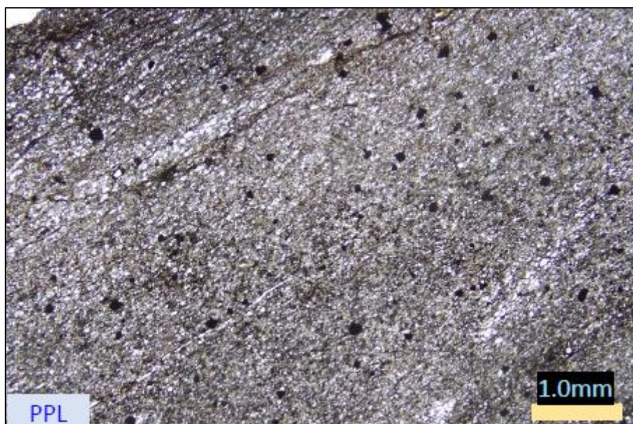
Figure 6: Sample DDBH031 (57-58 metres) from HWAC207: Sanukitoid intrusion – very fine grained quartz biotite schist. Disseminated small former pyrite cubes now replaced by Fe oxy-hydroxides (black inclusions).
