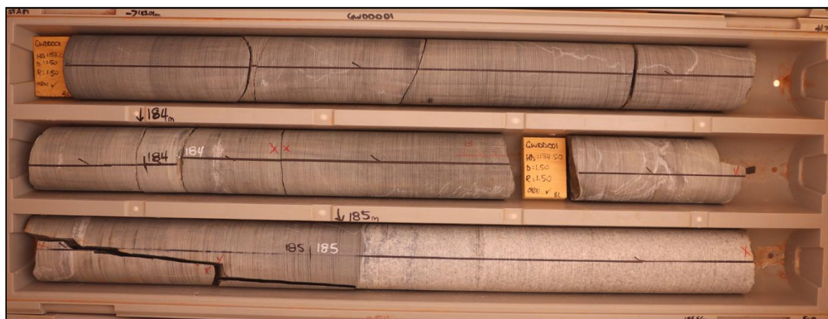
Figure 4: GWDD001 Diamond drill core highlighting the sediment-granite contact at 185.1 metres. 1
